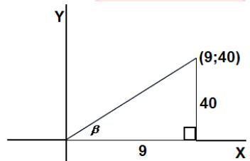
$$\begin{aligned}x^2 + y^2 &= r^2 \\(9)^2 + (40)^2 &= r^2 \\81 + 1600 &= r^2 \\r^2 &= 1681 \\r &= 41\end{aligned}$$
