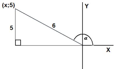
$$\begin{aligned}x^2 + y^2 &= r^2 \\x^2 + (5)^2 &= (6)^2 \\x^2 &= 36 - 25 \\x &= -\sqrt{11}\end{aligned}$$
