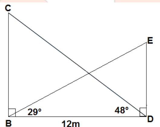
$$\begin{aligned}\Delta BCD : \\ \frac{BC}{BD} = \tan 48^\circ \\ \frac{x}{12} = \tan 48^\circ \\ x = 12 \times \tan 48^\circ \\ x = 13.33m\end{aligned}$$
