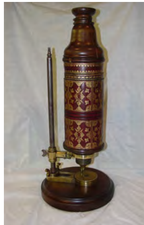
Robert Hooke's microscope that he used to first view cells.
