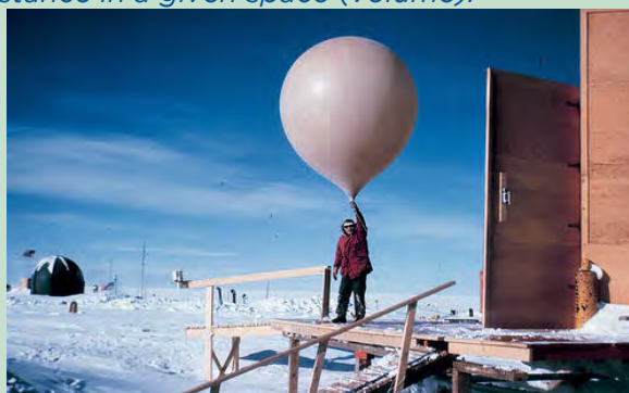
This man is about to launch a weather balloon filled with hydrogen gas. It will float upwards to collect information about the weather in Antarctica.
