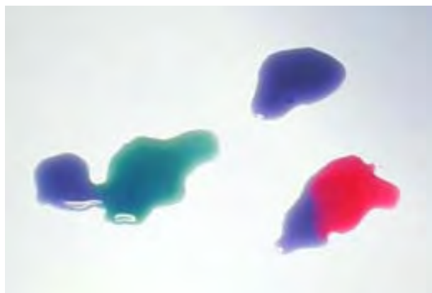
Red cabbage water mixed with base (left) and with acid (right). The blue drop at the top is the juice in a neutral solution (water).
