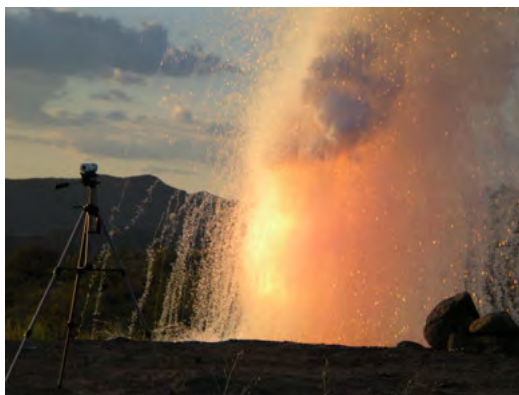
When large amounts of sodium come into contact with water, there is an explosion, such as in this photo where water was poured on 1,5 kg of sodium.
