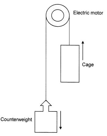
The cage, carrying passengers, moves vertically upwards at a constant speed, covering 60 m in 2 minutes. The counterweight has a mass of 900 kg. The total mass of the cage and passengers is 1 300 kg. The electric motor provides the power needed to operate the lift system. Ignore the effects of friction.
