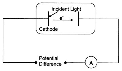
The incident light has an energy of 2,12 x  $10^{-18}$  J and the cathode has a threshold frequency of 2,21 ×  $10^{15}$  Hz.
