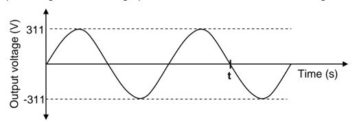
The output voltage is generated at a frequency of 50 Hz.
