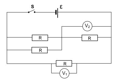
When switch **S** is CLOSED, the reading on voltmeter  $V_1$  is 3 V.
