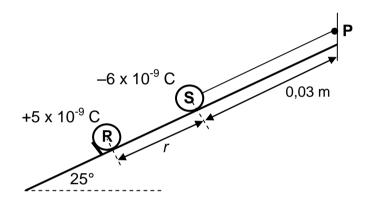
Sphere **R** exerts an electrostatic force of magnitude 1,2 x 10<sup>-3</sup> N on sphere **S**.
