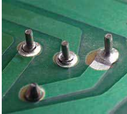
Broken solder joints on a flyback transformer
