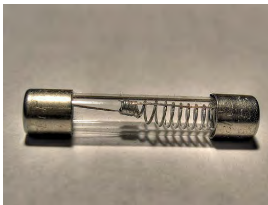
An example of a fuse. Can you see the low melting point wire inside?
