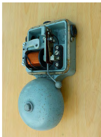
An electromagnet in a bell.
