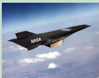
NASA's scramjet the X-43 flies at 7000 km/h.
