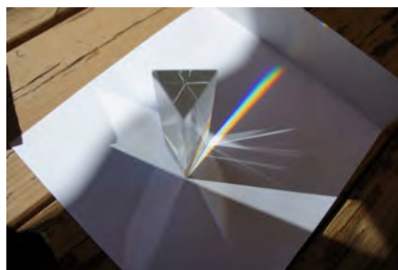
Refraction through a triangular prism.
