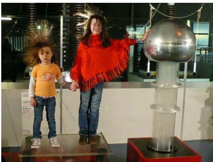
These girls are touching the large dome of a Van de Graaff generator.
