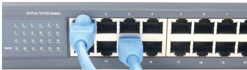
Figure 9.1: Switches allow multiple computers to connect to the same network
