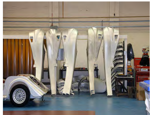
Can you see some parts of a car hanging up inside a car factory? These are made of sheets of metal.
