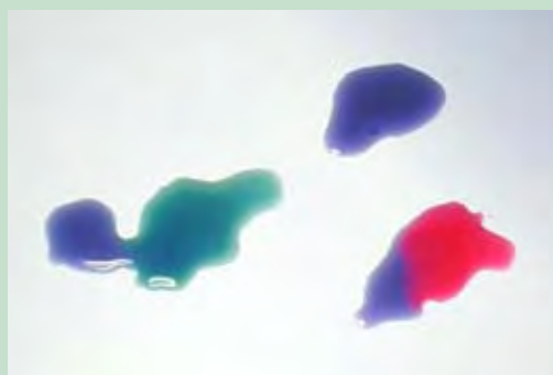
Red cabbage juice mixed with baking soda (left) and with vinegar (right). The blue drop at the top is the unmixed juice.
