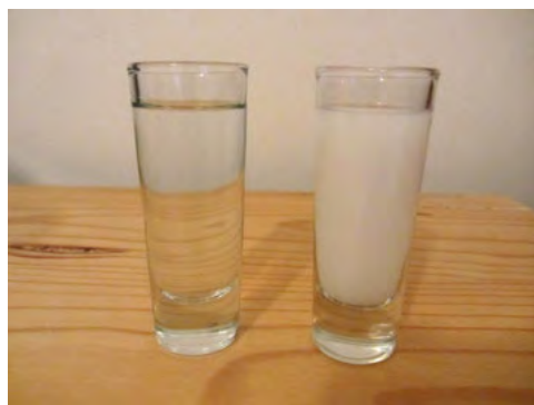
A clear, transparent solution on the left and an opaque emulsion on the right
