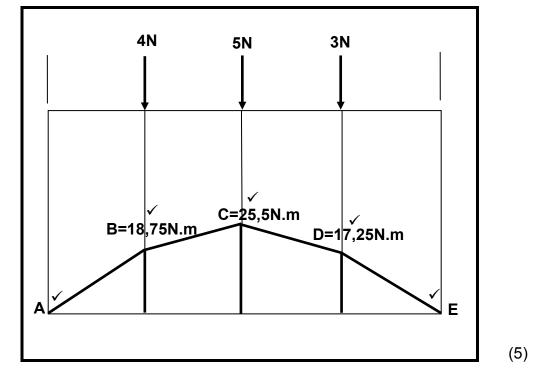
**SCALES:** Space diagram:10 mm = 1 m Bending moment diagram:5 mm = 1 N.m
