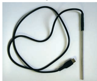
Figure 16.11e A temperature sensor containing a thermistor
