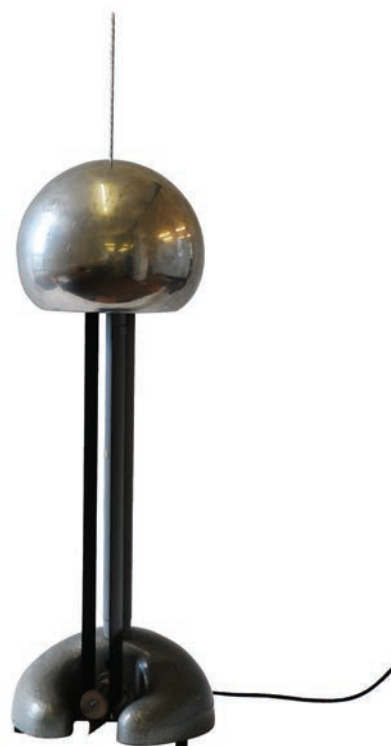
Figure 12.21 When the lightning rod is on top of the dome, electric charges can't build up.
