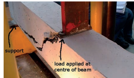
Figure 5.24 Shear cracks in a concrete beam – they start at the support.
