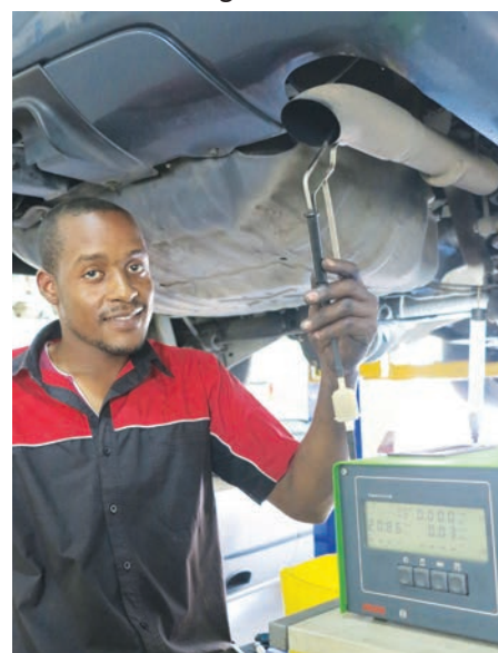
Figure 9.7 You might test exhaust gas to measure the percentage of carbon monoxide in the gas.
