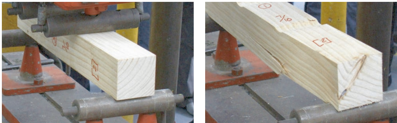
Figure 5.25 Shear in this piece of wood probably started when the fibres at the bottom of the beam failed in tension.
