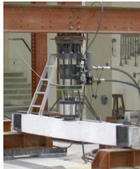
Figure 5.4 The concrete beam has failed at its midpoint.
