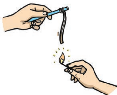
Figure 10.6 Wrap the magnesium around a pencil and heat the end of the magnesium.
