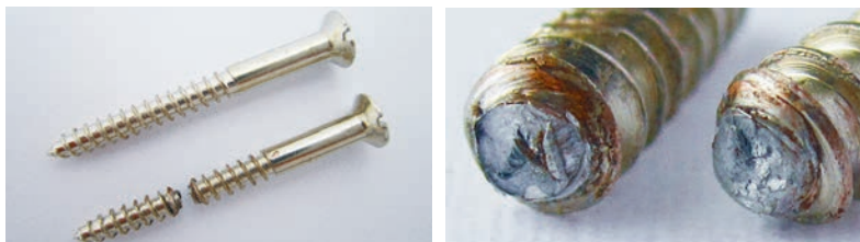
Figure 3.30 The two faces of a screw that has failed in torsion
