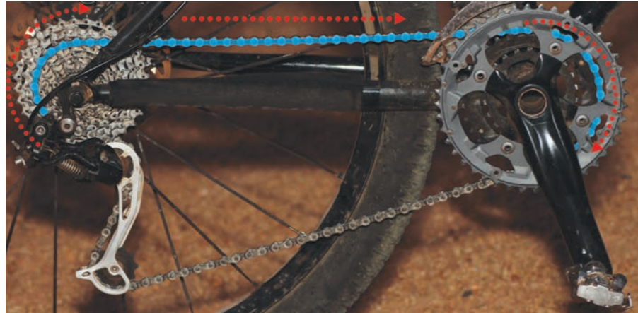
Figure 12: The back wheel of a bicycle is driven by the gear and chain mechanism
