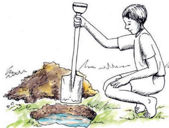
Figure 5: Holes dug in the ground often go below the water table, and then the hole fills with water.
