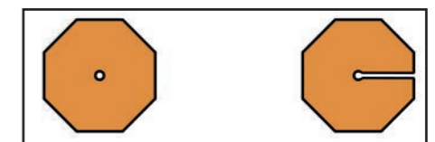
Figure 11: Spacers to use on axles
