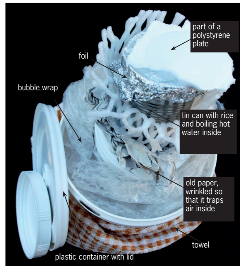
Figure 15: Insulated cooking box made of waste materials
