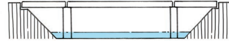
A beam-and-column bridge
