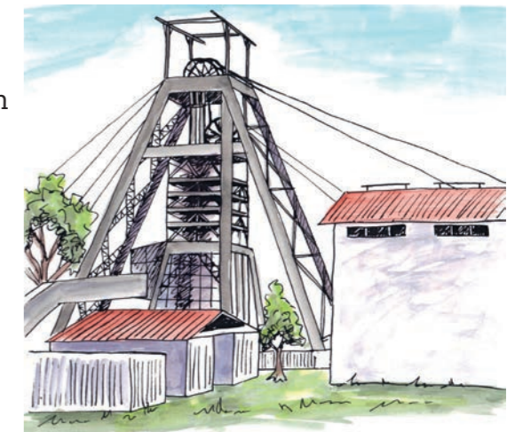
Figure 4: The headgear of an underground mine. The shaft goes straight down into the ground under the wheels of the headgear, sometimes kilometres deep.
