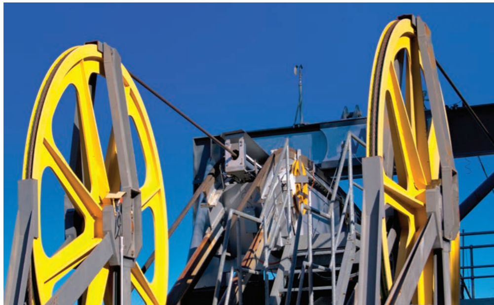
Figure 2: This photograph shows detail of sheave wheels used for pulling in a cable. The sheave wheels in the photograph are used for a cable car, but they are similar to the sheave wheels used on a mine's winch system.
