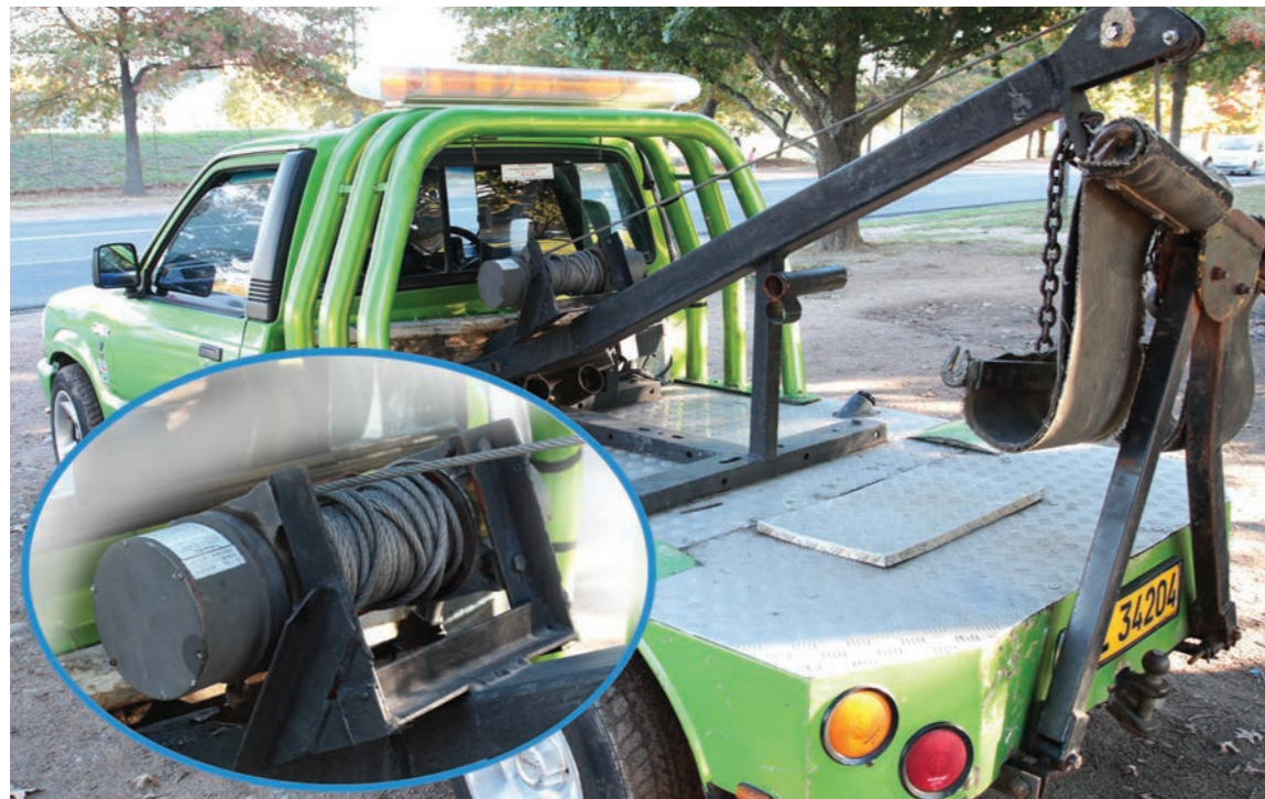
Figure 1: The back of a tow truck showing the winch that is used to lift and pull cars that have broken down. This winch is driven by an electric motor. It uses a gear system that gives a mechanical advantage.
