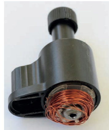
Figure 5: The exposed copper coils in a dynamo
