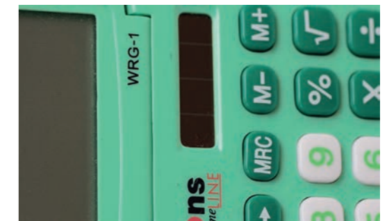
Figure 15: Photovoltaic cells in a calculator
