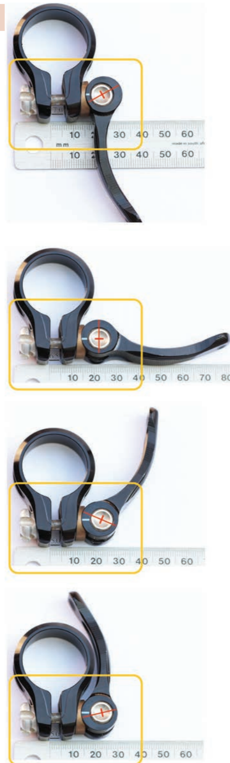
Figure 13: The sides of the quick-release mechanism move or clamp closer together as the eccentric cam is turned by the handle.
