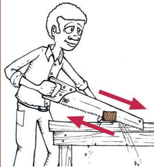
Figure 1: When you saw wood you make a reciprocating movement.
