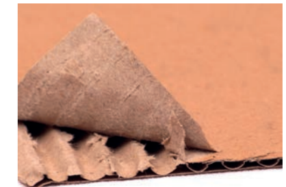
Figure 11: Large boxes are made of corrugated cardboard.
