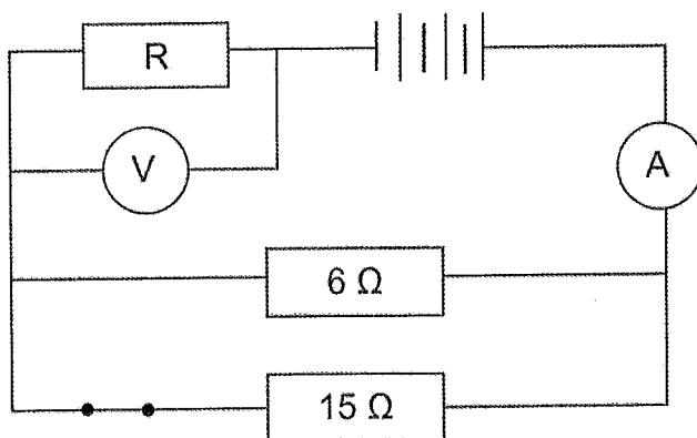
The total power dissipated in the parallel part of the circuit is 50 W.
