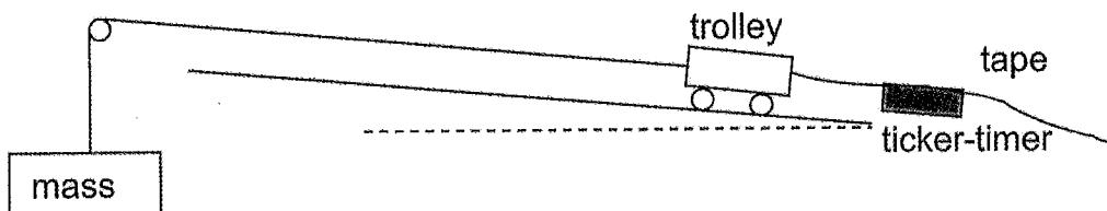
(1) Ticker-tape attached to the trolley passes through the ticker-timer. The acceleration of the trolley is determined by analysing the ticker-tape. The results of the net force produced by the different masses and the acceleration of the trolley were recorded in the table below.
