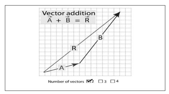
The picture below shows a force diagram of the addition of two vectors.
