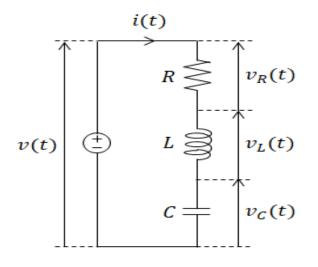
The diagram below models an AC circuit with two impedances,
