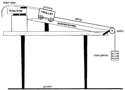
The runway was gently tilted as individual mass pieces were added onto the trolley whilst a constant force acted on the system. The results obtained were used to plot the graph shown.
