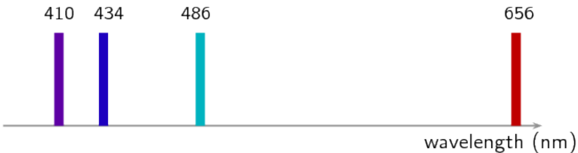
Figure 7: Diagram of the emission spectrum of hydrogen in the visible spectrum. Four lines are visible, and are labelled with their wavelengths. The three lines in the 400–500nm range are in the blue part of the spectrum, while the higher line (656nm) is in the red/orange part.
