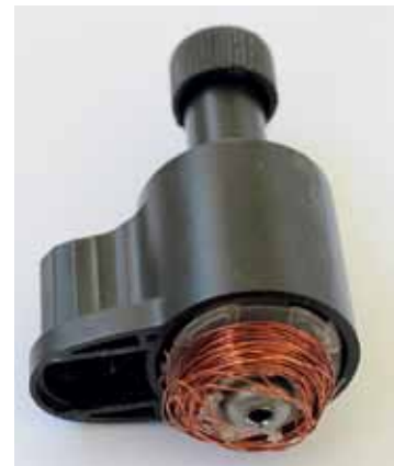
Figure 5: The exposed copper coils in a dynamo
