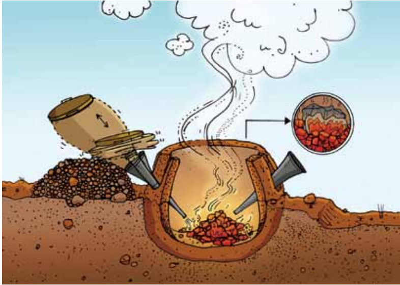
Figure 12: Illustration of how an early iron smelter was constructed and used
