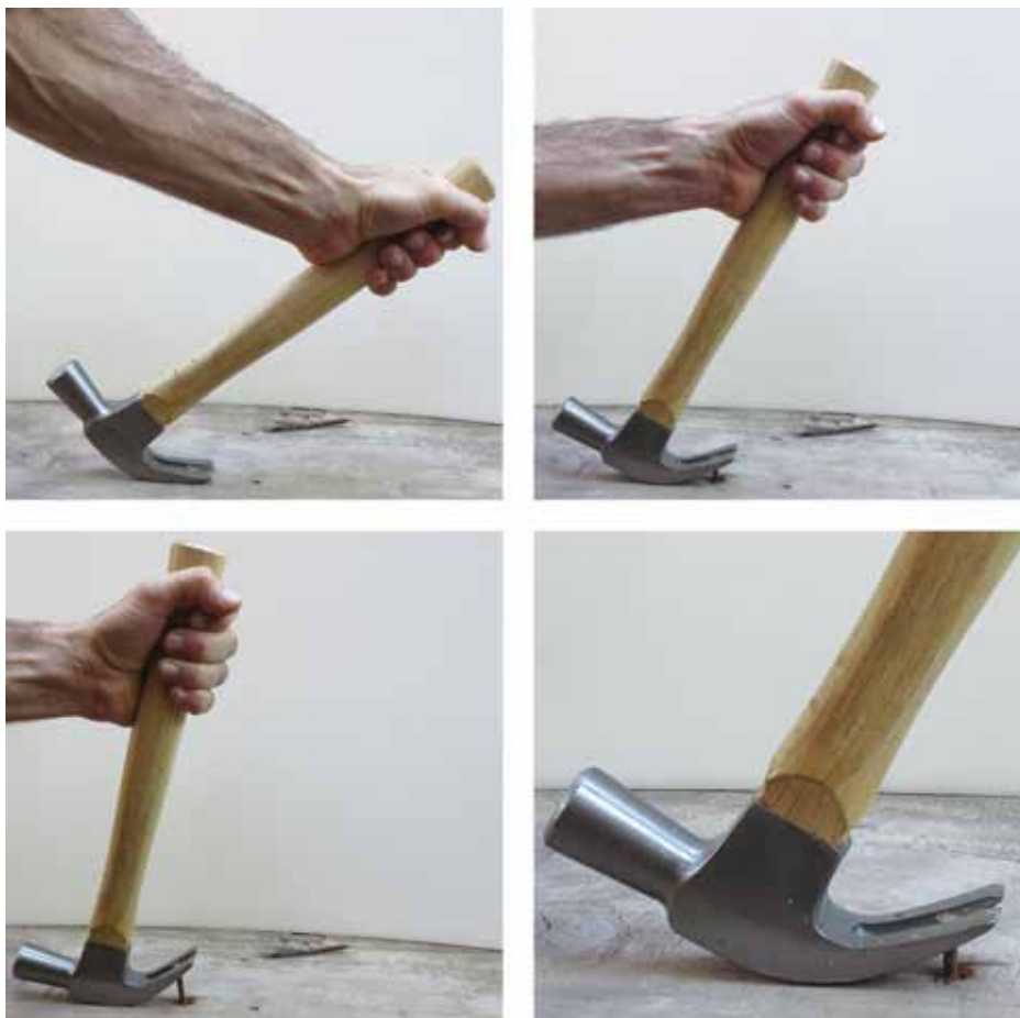
Figure 1: A claw hammer can be used as a lever to remove nails from wood.
