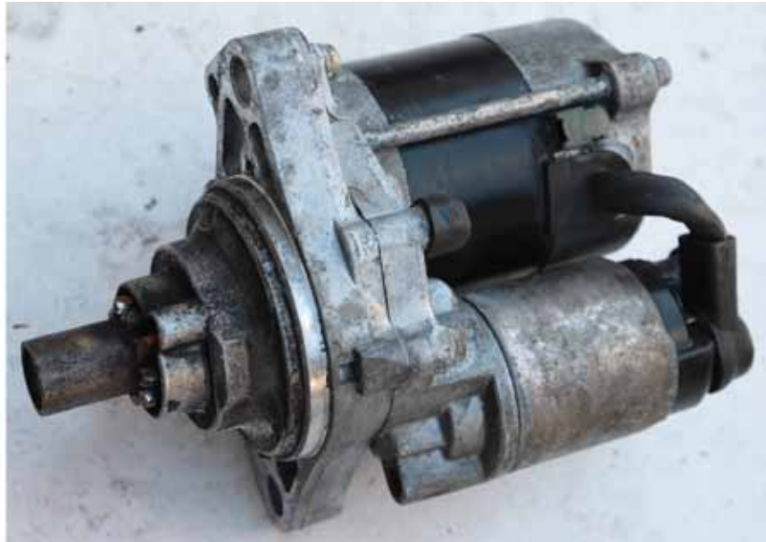
Figure 6: A car's starter motor has a small driver gear called a pinion, which is used to turn a bigger gear on the engine.
