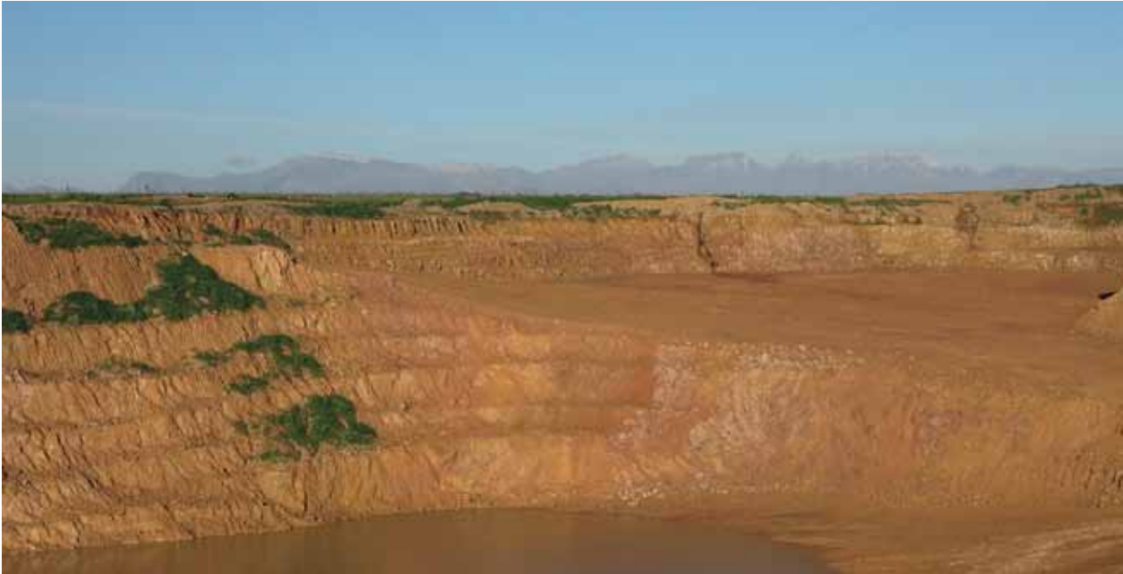
Figure 3: An opencast or surface mine. Note the water collecting in the hole.
