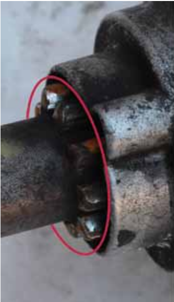
Figure 6: A car's starter motor has a small driver gear called a pinion, which is used to turn a bigger gear on the engine.
