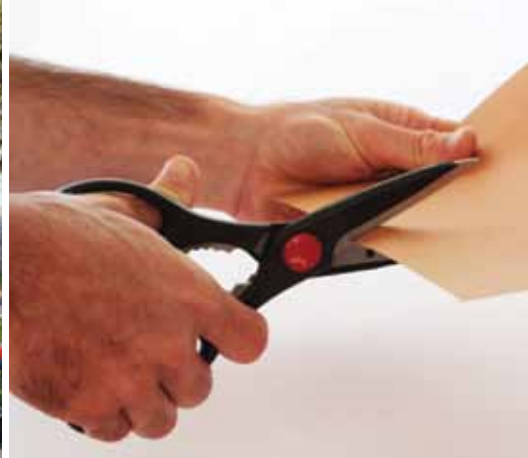
Figure 16: A pair of scissors is a pair of linked first-class levers.
