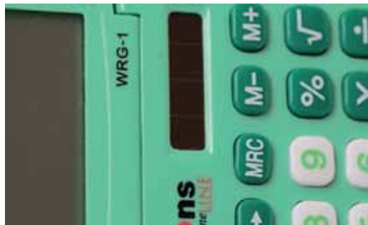
Figure 15: Photovoltaic cells in a calculator
