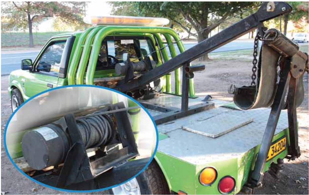
Figure 1: The back of a tow truck showing the winch that is used to lift and pull cars that have broken down. A winch is a gear that gives a mechanical advantage. You will learn about winches in this chapter.
