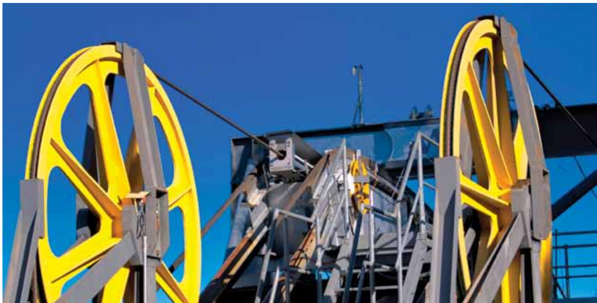
Figure 2: This photograph shows detail of sheave wheels used for pulling in a cable. The sheave wheels in the photograph are used for a cable car, but they are similar to the sheave wheels used on a mine’s winch system.
