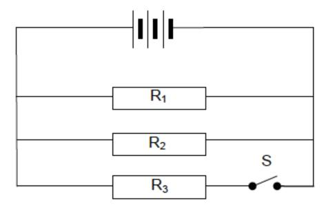
When switch **S** is closed, which one of the following correctly describes the change in total current and total resistance in the circuit?
