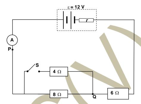
With switch **S OPEN**, ammeter A gives a reading of 0,8 A.
