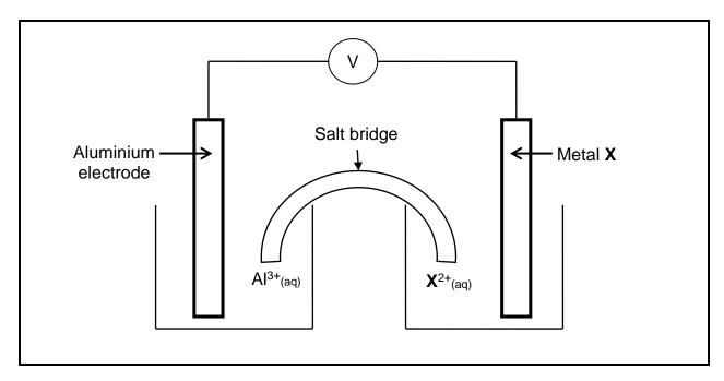
In the external circuit, electrons flow from the aluminium electrode to metal X. Under standard conditions, the initial voltmeter reading is 1,52 V.
