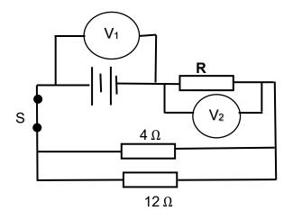
The total power dissipated in the parallel part of the circuit is 50 W. The voltmeter across resistor  $\mathbf{R}$  reads 8 V.
