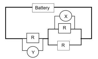
If voltmeter Y records a potential difference of V, then the reading on voltmeter X would be ...
