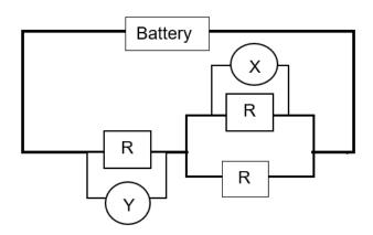
If voltmeter  ${\bf Y}$  records a potential difference of  ${\bf V}$ , then the reading on voltmeter  ${\bf X}$  would be ...
