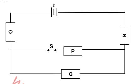
Switch S is now OPENED. Which ONE of the following combinations of changes will occur in O, Q and R?
