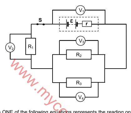
Which ONE of the following equations represents the reading on voltmeter V<sub>1</sub> in terms of the readings on the other voltmeters? 200.CO.49
