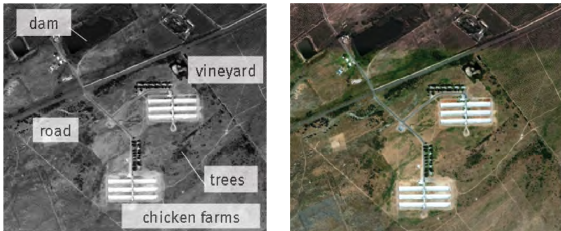
FIGURE 13 Shape and pattern are used to distinguish between objects on both panchromatic and colour photographs.
