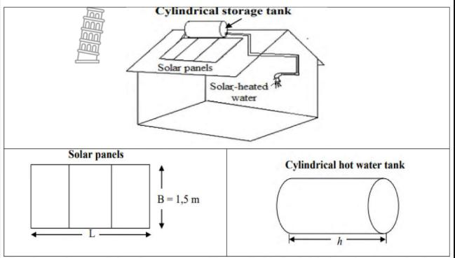
The solar panels use sunlight to heat water stored in the cylindrical tank. The heated water can then be used in the house. There are altogether six people in Elvis Louw's household.
