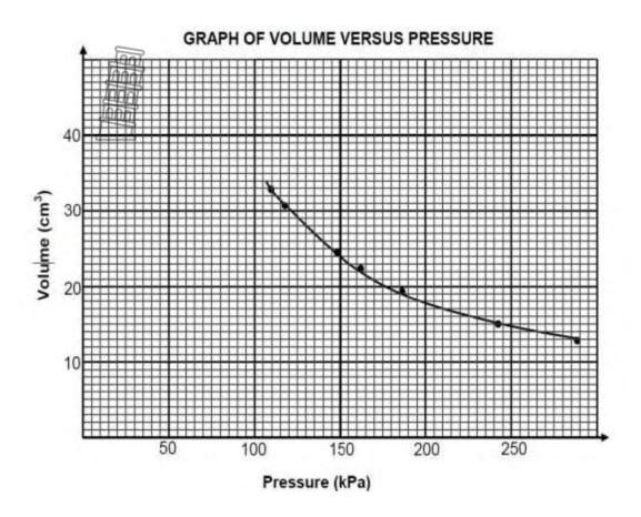
A fixed mass of oxygen is used to verify one of the gas laws. The results obtained are shown in the graph below.
