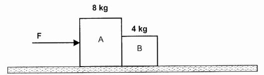
A horizontal force of magnitude F is applied to box A and the system accelerates uniformly to the right. The net force acting on block B during its motion is 12.5 N and the coefficient of kinetic friction between each block and the surface is 0.2. Take the motion of the system to the right as positive.
