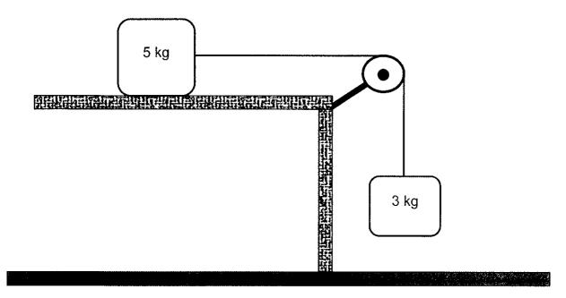
The kinetic friction between the 5 kg mass and the surface is 4.5 N.
