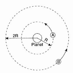
distances of satellites A and B from the centre of the planet are R and 2R respectively,if gravitation force that the planet exerts on A is F, then the gravitational force that the et exerts on B will be
