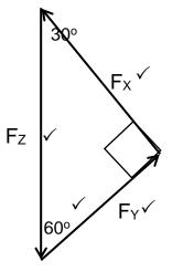
$\begin{array}{l} F_x \text{-} \text{ Force in string X} \\ F_y \text{-} \text{ Force in string Y} \\ F_z \text{-} \text{ Force in string Z / Weight} \end{array}$
