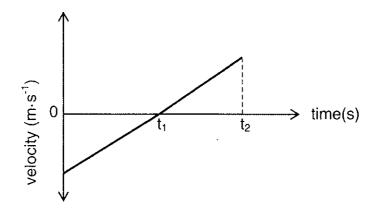
Which ONE of the following statements BEST describes the magnitude of the force exerted by the car's engine from t = 0 to  $t = t_2$  seconds?
