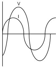
Shape of voltage waveform larger than current waveform ✓ Phase difference showing current leading voltage ✓ (2)
