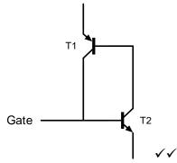
'+' pulse on the gate switches TR2 on causing collector of TR2 to become more negative. ✓
