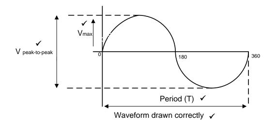
5.3  $f = \frac{1}{T} \checkmark$ =  $\frac{1}{10 \times 10^{-3}} \checkmark$ = 100 Hz  $\checkmark$  (3)
