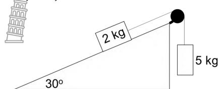
The coefficient of kinetic friction between the wooden block and the metal plane is 0,3.
