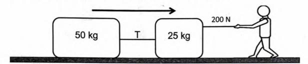
The crates move with an acceleration of 1,25 m·s<sup>-2</sup> to the right across a rough horizontal surface. The coefficient of kinetic friction is the same for both crates.
