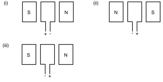
Which of the changes to the motor above will change the original direction of rotation of the coil?
