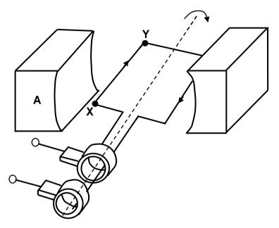
When the coil of the generator rotates clockwise between the two poles of the magnet, the direction of the induced current is from **X** to **Y**, as shown above.
