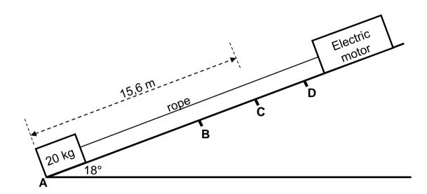
The motor exerts a constant force of 96,8 N parallel to the inclined plane on the rope.
