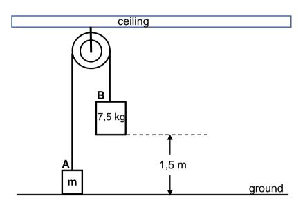
When block **B** is released, it moves vertically downwards and strikes the ground with a velocity of  $3,41 \text{ m}\cdot\text{s}^{-1}$ .
