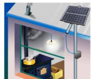
Figure 22 In this picture, you can see a solar panel. It uses energy from the Sun to make electricity. The energy can be stored in the battery and is used for lighting at night
