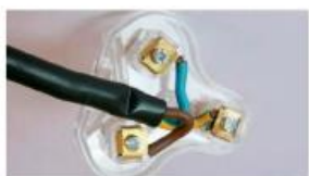
Figure 4 Wiring inside a three-pin plug
