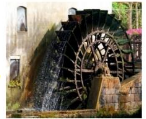
Figure 18 A water-wheel. Moving water pushes the wheel around. In a watermill, water wheels are used to help grind grain to make flour
