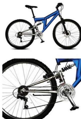
Figure 1 The cyclist puts energy into the system by pushing the pedals. The pedals transfer the energy through a chain to the back wheel. The energy is changed to movement energy and the bicycle moves
